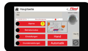
Fig. 13: PLC machine control unit
