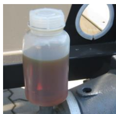
Fig. 16: Oil container for lubricating the flushing pump
